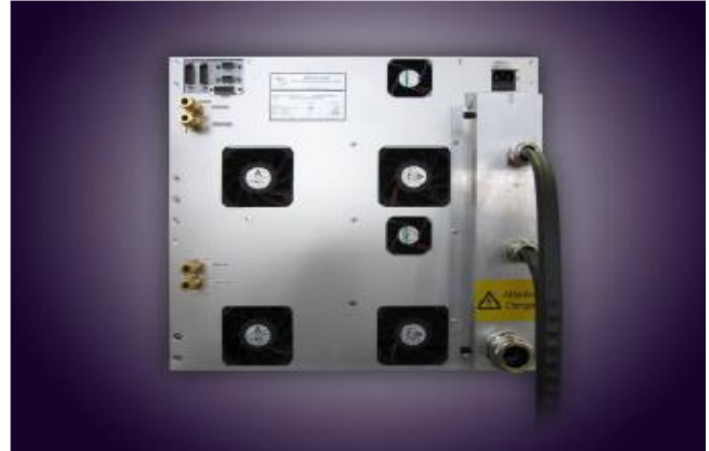
Rear side with connecting cables
